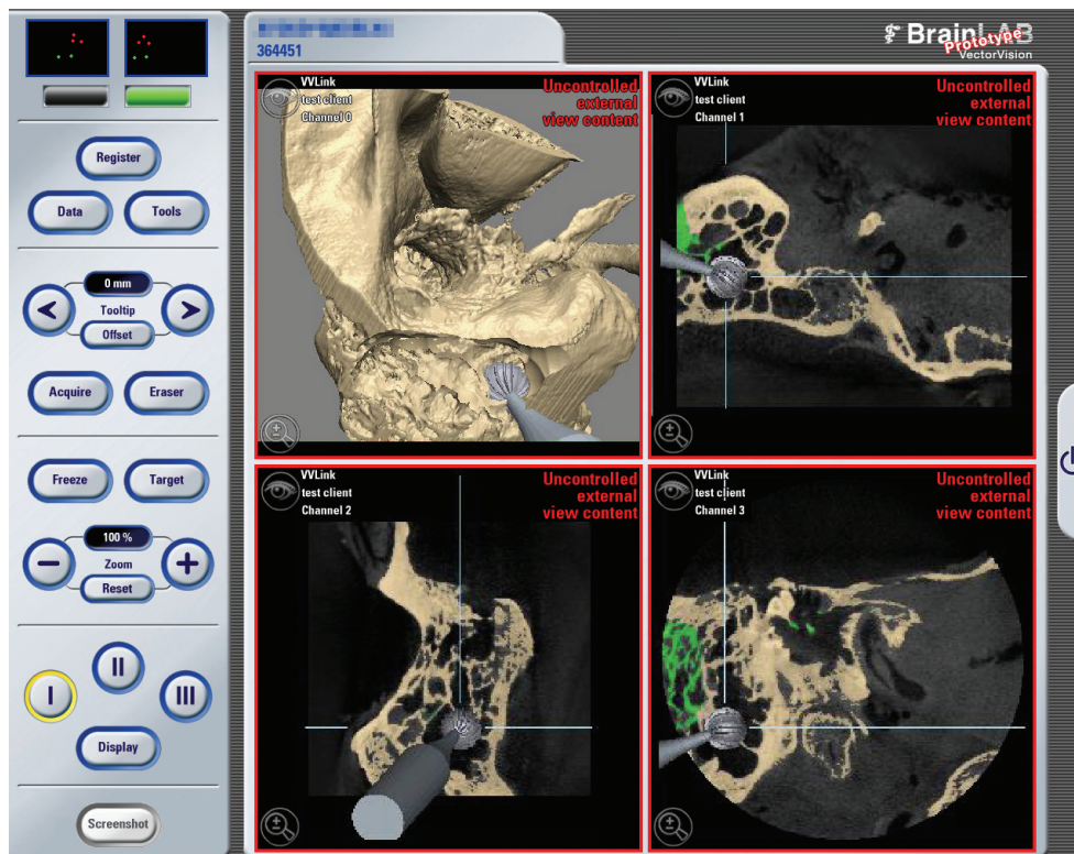
Figure 4: Screenshot of the VectorVision surgical navigation system, connected to the simulator. The 3D views and cross-sectional images uploaded from the simulator indicate the workspace as defined during surgery planning and rehearsal, and may thus easily be accessed in the operating room.
